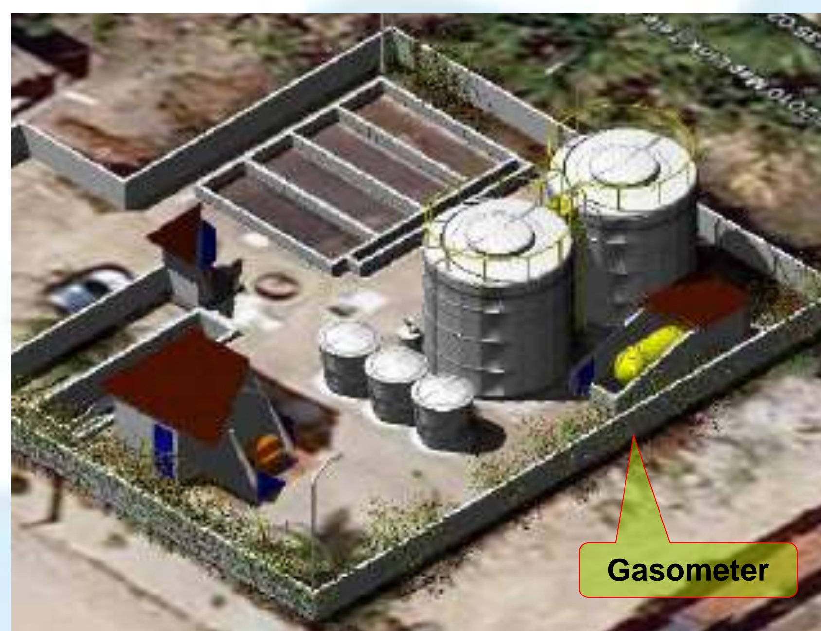
Figure 1. Figures showing the two UASB reactors, as well as generator, pump station and storage of biogas.
