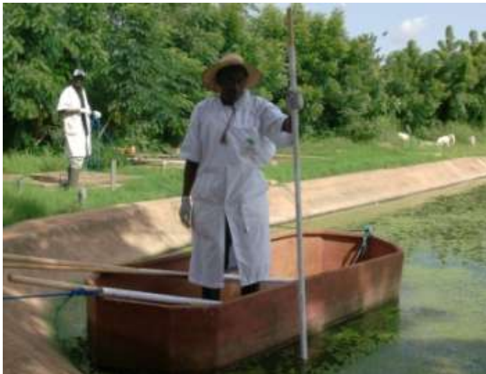
Pre-prepared grid of Ponds for Bathymetric surveys of sludge accumulation
