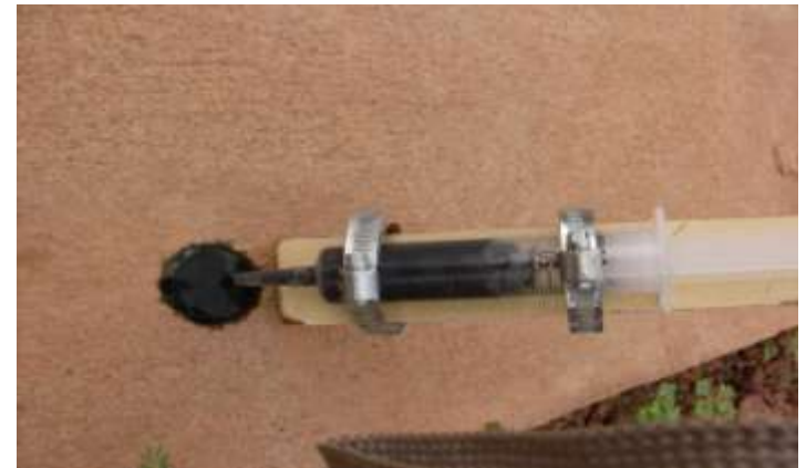
Device of shaft syringe for sludge sampling
